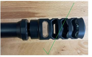
STEP #4 THREAD BRAKE ONTO BARREL ALIGNING IT TO DESIRED LOCATION. ENSURE THE THREADED BARREL END IS AS CLOSE TO FLUSH AS POSSIBLE WITH START OF THE FIRST SLOT. DO NOT THREAD PAST THE FIRST PORT SLOT
