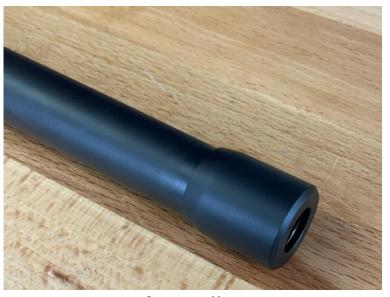
STEP #1 KEEP THREAD PROTECTOR ON UNTIL YOU HAVE DETERMINED THE CORRECT BULLET SIZE FOR YOUR BARREL. ONCE BULLET SIZE IS DETERMINED, PROCEED TO INSTALL PORTED BRAKE
